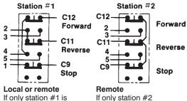
If only station #1 is used jumper C9-C11-C12 is used jumper C9-C11-C12 is used jumper C11-2, C12-4 & conn. C9-"1" at starter
