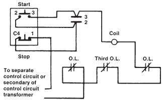
NOTE: If starter is wired with a jumper between L2 and overload relay contact, this jumper must be removed
