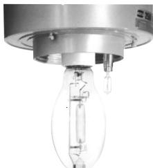
The quartz auxiliary lamp comes to full brightness instantly and remains lit until the H.I.D. lamp attains 60-70% of full illumination. Quartz auxiliary lamps can be used with all DMV, VMV and VMV high wattage series *Champ*® luminaires. Use for non-hazardous applications ONLY.
