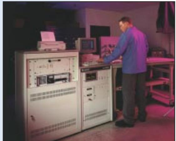
Automatic circuit analyzers (like the DIT-MCO 9500 and the Omni Tester) allow precise testing of cables, harnesses and sub-assemblies to 2,000 VDC/1,500 VAC to 2.5 Amperes. Can be configured to meet any user-specified requirement up to 100,000 test points.
