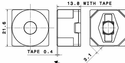
Space for D=5.0 mm screw head between the lenses for fastening of PCB
